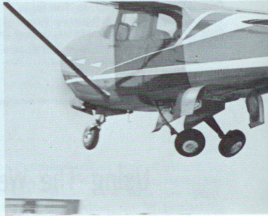
soaring bird, increase the airplane's spiral stability, Cessna says (3) Close-up of 210 gear. Note that all housing doors are closed on the ground as well as in the air. They open only during actual retraction or extension cycle. Rear wheels are on a single-piece spring steel gear popularized by Cessna. This is the first time this type of gear has been made retractable (4) This view of the 210 taking off shows how landing gear performs; nose wheel goes forward, main wheels inward and backward. All the open doors close flush
